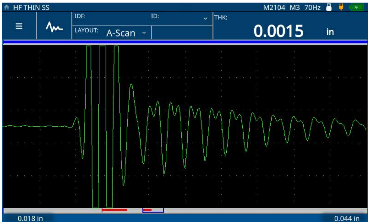
72DL PLUS gauge measures thin steel (0.0015 in. or 0.0381 mm) using the M2104 (125 MHz) transducer
